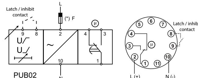
Connect the power supply to the proper terminals.
