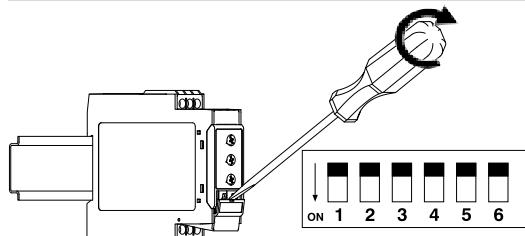
Adjust the input range setting the DIP switches 5 and 6. Select the desired function setting the DIP switches 1 to 4.
