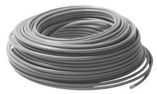
The grey Danfoss FH composite pipe is 100% impervious to air, temperature resistant and highly flexible. It consists of an aluminium pipe which is covered inside and out with a cross-linked Polyethylene layer.
