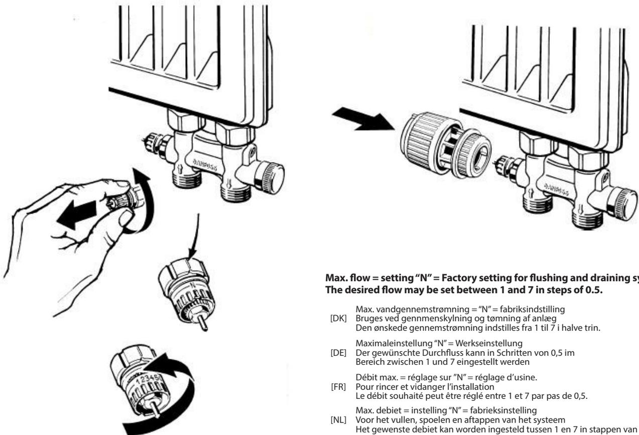
**Max. flow = setting "N" = Factory setting for flushing and draining system
