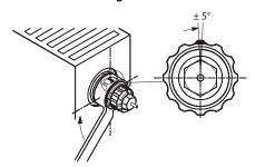
An integrated valve can only be fitted once in a radiator (because of the load on the deformation zone).
