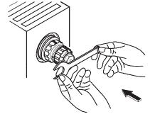
While the system is in operation, the gland seal can be replaced by means of a spanner, KW 10. Hold the setting ring using a 12-edge ring-spanner, KW 17.
