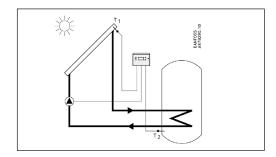
T1: Temperature sensor in solar collector
