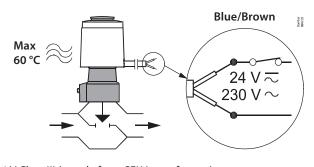
24 V Class III (supply from SELV transformer) 230 V max. 3 A pre-fuse
