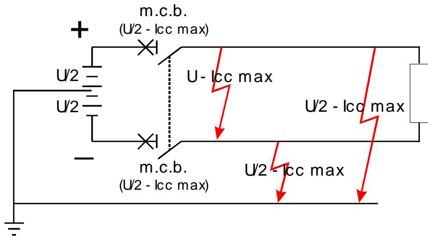
Example : installation connected to the earth by the middle / U = 180 V DC / Icc = 6 kA / In = 10 A
