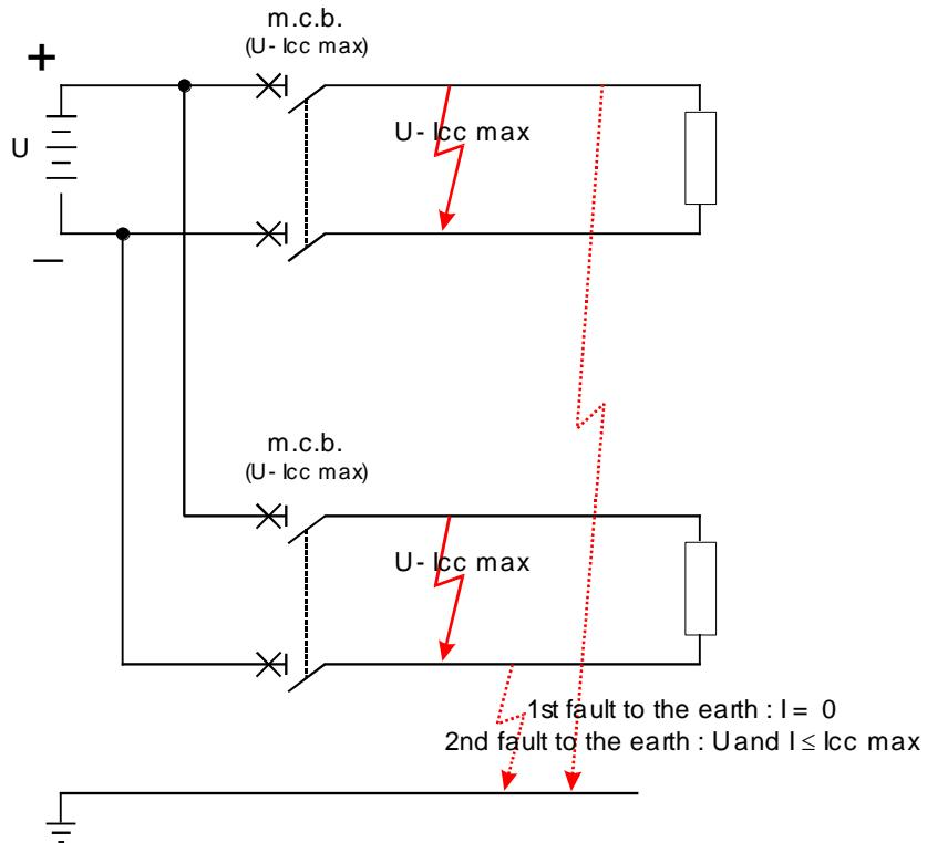
Example : installation isolated from the earth /  $U = 48 \text{ V DC} / I_{cc} = 6 \text{ kA} / I_n = 40 \text{ A}$
