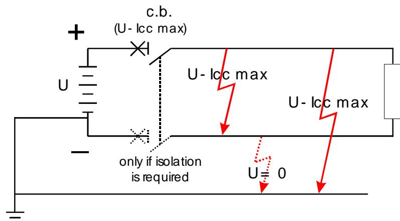
Example : installation connected to the earth by the negative polarity /  $U = 110 \text{ V DC} / I_{cc} = 10 \text{ kA} / I_n = 32 \text{ A}$
