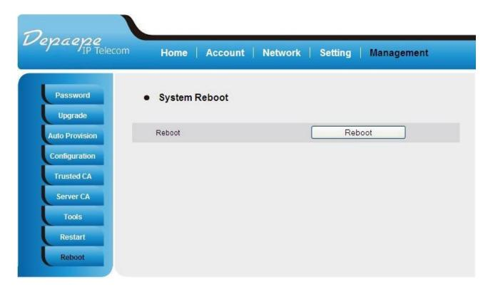
You can reboot the HD2000IP by clicking on the "Reboot" button after each update to the configuration page. Alternatively, you can reboot by unplugging the power supply of the HD2000IP and then powering it on again. If your HD2000IP ever becomes "stuck" or un-responsive, you can unplug the power supply to reboot it. Frequent rebooting by unplugging the power supply is not recommended and should not be necessary.
