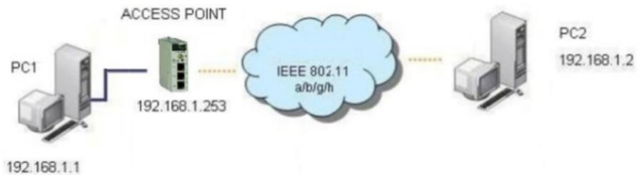
Setup PC2 Wireless network interface according to the default parameters of the ACKSYS AP device (802.11b/g, SSID ACKSYS, no security).
