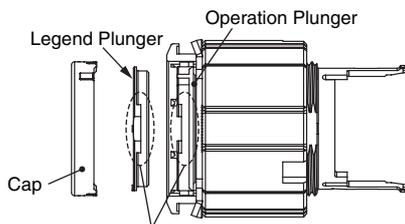
Insert the legend plunger so that the groove widths are lined up.
