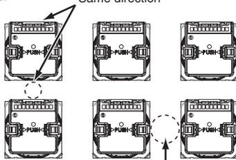
Allow space between switches for fingers to push locking levers..
