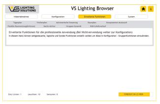
The "Advanced Functions" menu item contains useful additional functions with which luminaire groups can be controlled, system architecture can be displayed or maintenance functions can be optimised. These must subsequently be integrated into the "Group Functions" menu.
