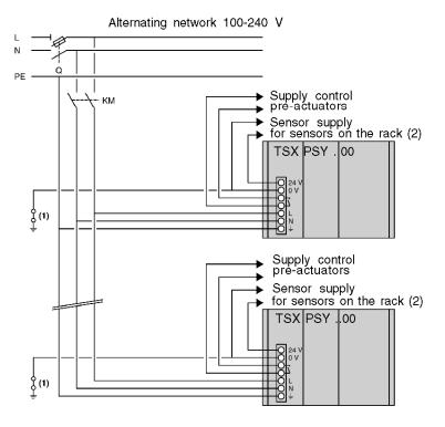
**NOTE:** If there are several PLC stations supplied by the same network, the principles of connection are identical.
