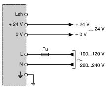
Fu=External safety fuse on phase (Fu): 250 V 4 A time delay
