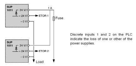
**NOTE:** TSX SUP 1051 and 1101 suppliers are not equipped with a serial diode, which is required for the redundancy function.
