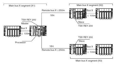
Taking this into account, the maximum distance possible between the processor and the remote modules is 350 meters.
