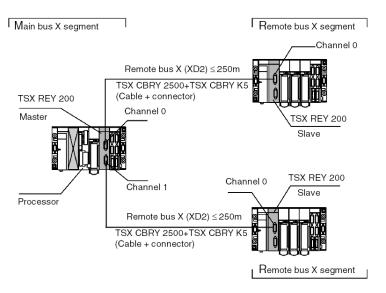
NOTE: Each bus X segment must have a A/ and B/ line terminator (see page 396)at each end.
