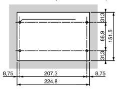
(1) The diameter of the fixing holes must be suitable for M6 screws.
