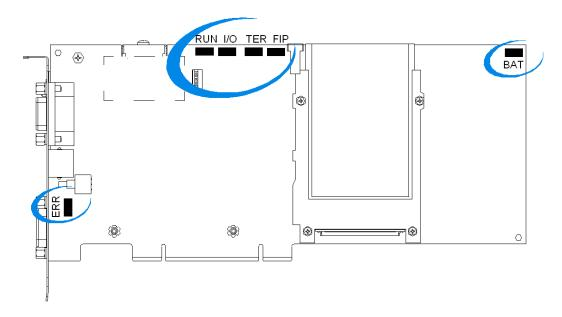
Due to the small amount of space available on the shield, only the ERR LED is visible when the PC housing the processor is closed.
