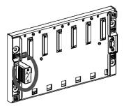
TSX TLYEX line terminations are sold in twos and marked **A**/ and **/B**. The bus must be fitted with a terminator **A**/ at one end and a terminator **/B** at the other end in no predefined (see page 397) order.
