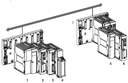
**NOTE:** If the second rack does not contain a processor module, this is a **single** PLC station distributed on 2 racks.
