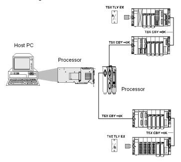
**NOTE:** In this case, since the processor is no longer integrated at the start of the line terminations **TSX TLY EX A/** and **/B** must be installed on each of the racks located at the end of the line.
