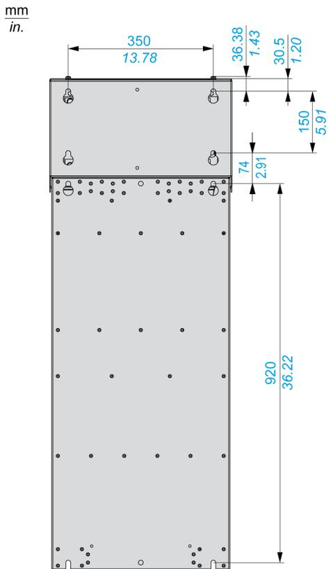
**NOTE:** Lower Conduit Box part sold separately. This part enables wall mounting of the product. It provides IP21 protection degree on the bottom side and UL type 1 protection degree.
