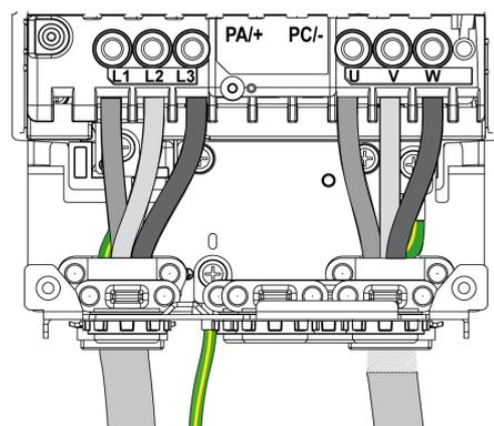
**NOTE:** PA/+ and PC/- terminals are used only to measure the DC Bus voltage and are not intended to be wired for an external use.
