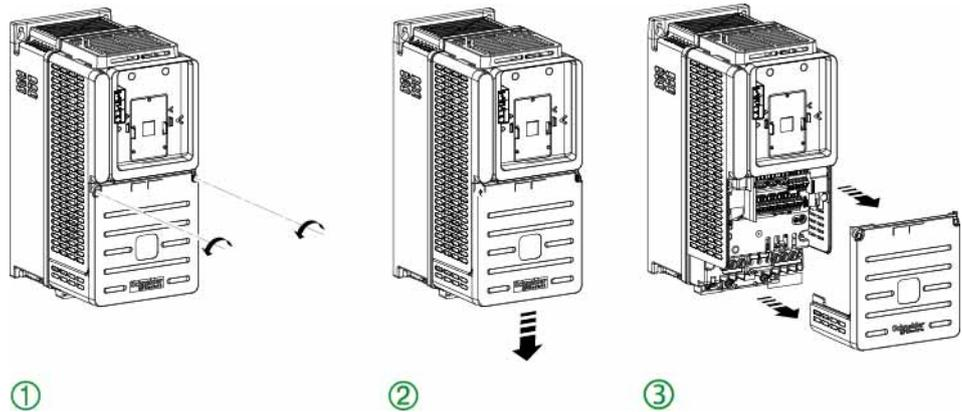
Apply the following instructions to access the terminals on **frame sizes 1 to 3** IP20 drives
