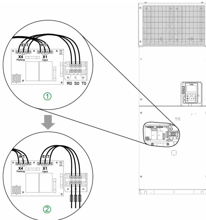
① Factory wiring: Fans powered internally by R/L1, S/L2, T/L3.
