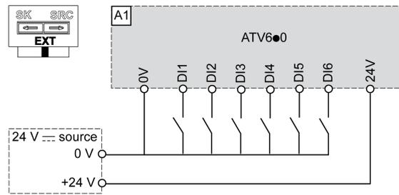
Switch set to **EXT** (Sink External) position **with functional isolation** on digital inputs. This configuration requires the use of 2 external supply units.
