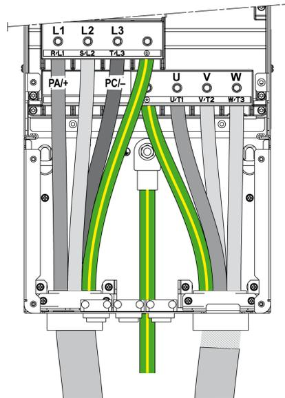
**NOTE:** PA/+ and PC/- terminals are used only to measure the DC Bus voltage and are not intended to be wired for an external use.
