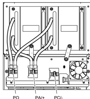
**NOTE:** PA/+ and PC/- terminals are used only to measure the DC Bus voltage and are not intended to be wired for an external use.
