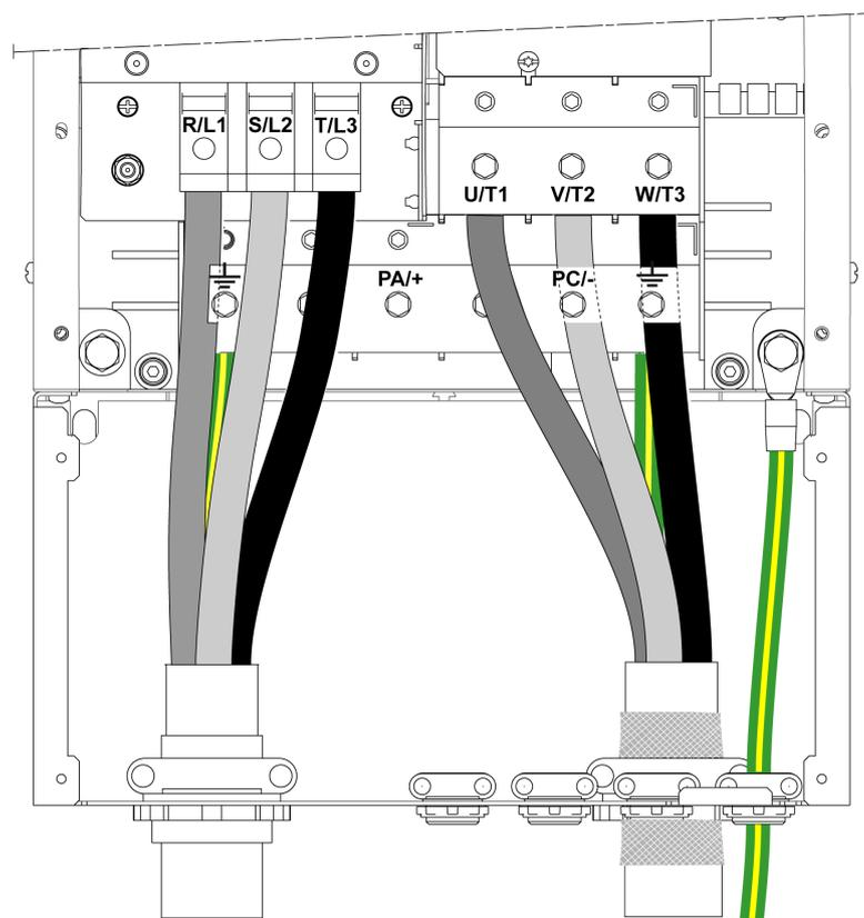
**NOTE:** PA/+ and PC/- terminals are used only to measure the DC Bus voltage and are not intended to be wired for an external use.
