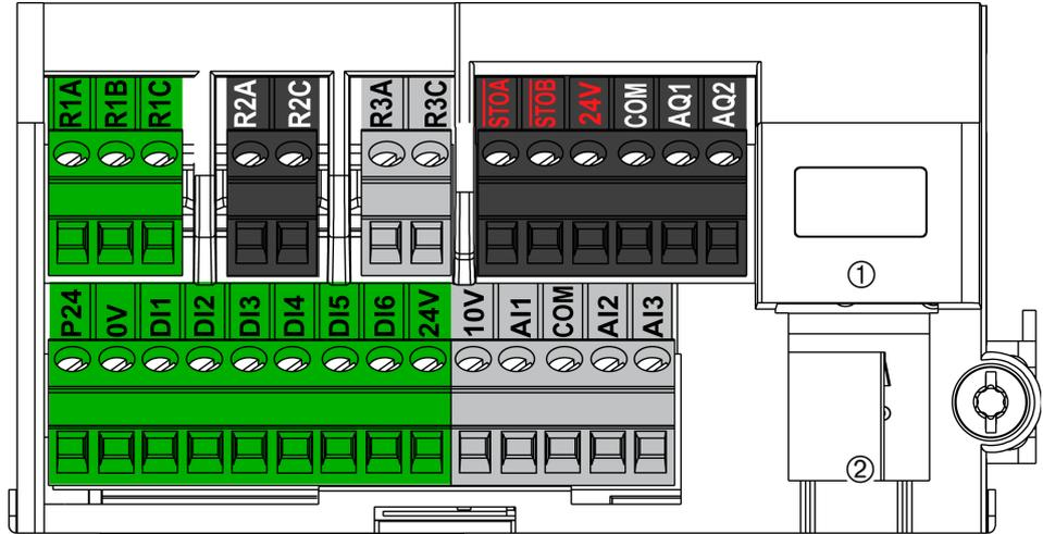
① Ethernet Modbus TCP, ② Serial Modbus
