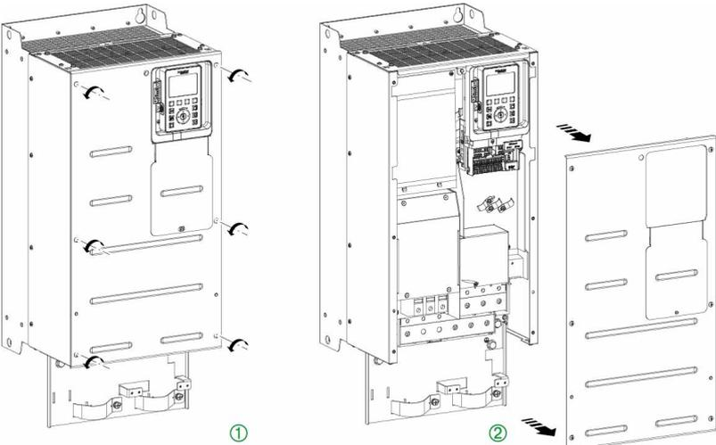
Apply the following instructions to access the terminals on **frame sizes 3Y and 5Y** drives
