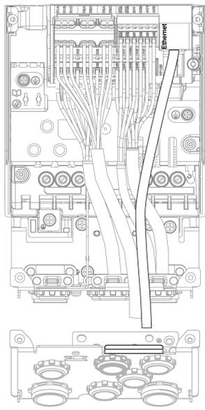
**NOTE:** Cabling plate shown is for frame size 2. Other cabling plates look slightly differs from this one.
