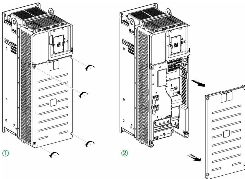
Apply the following instructions to access the terminals on **frame sizes 4 and 5** drives
