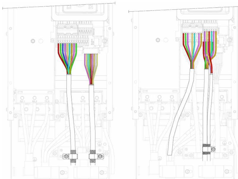
Example: cable path for frame size 5Y for 500-690 V mains voltage
