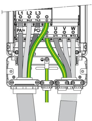
**NOTE:** PA/+ and PC/- terminals are used only to measure the DC Bus voltage and are not intended to be wired for an external use.
