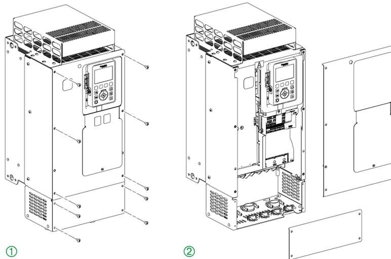
Apply the following instructions to access the terminals on **frame sizes 3S and 5S** drives
