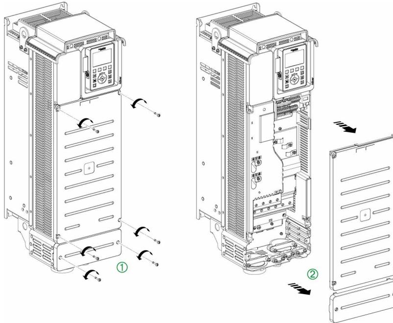
Apply the following instructions to access the terminals on **frame sizes 4 and 5** drives
