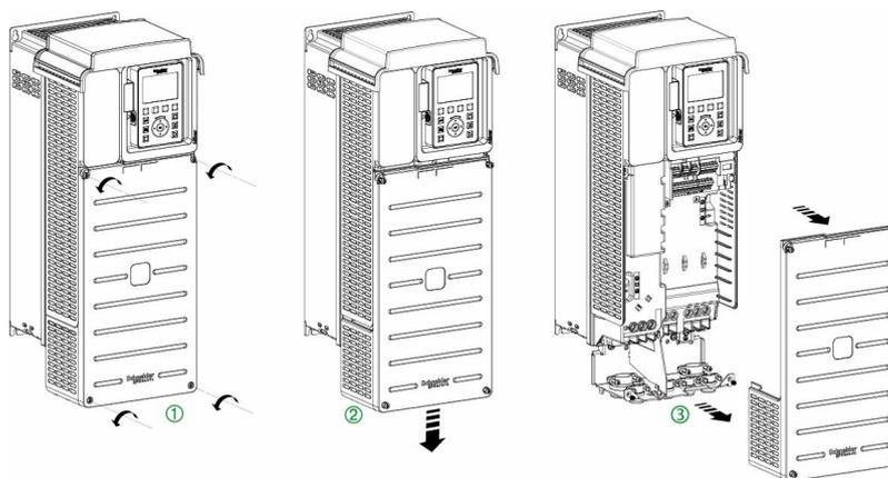
Apply the following instructions to access the terminals on **frame sizes 1 to 3** drives
