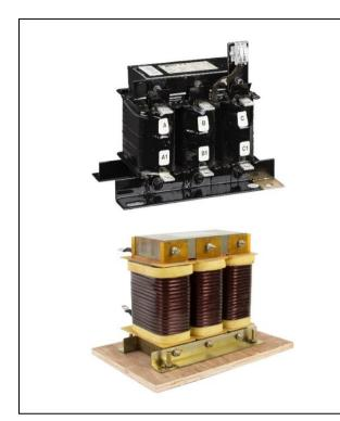
Both PowerLogic PFC Detuned Reactors and EasyLogic PFC Detuned Reactors should be associated with capacitor banks for Power Factor Correction in systems with significant non-linear loads, generating harmonics. Capacitors and reactors are configured in a series resonant circuit, tuned so that the series resonant frequency is below the lowest harmonic frequency present in the system.
