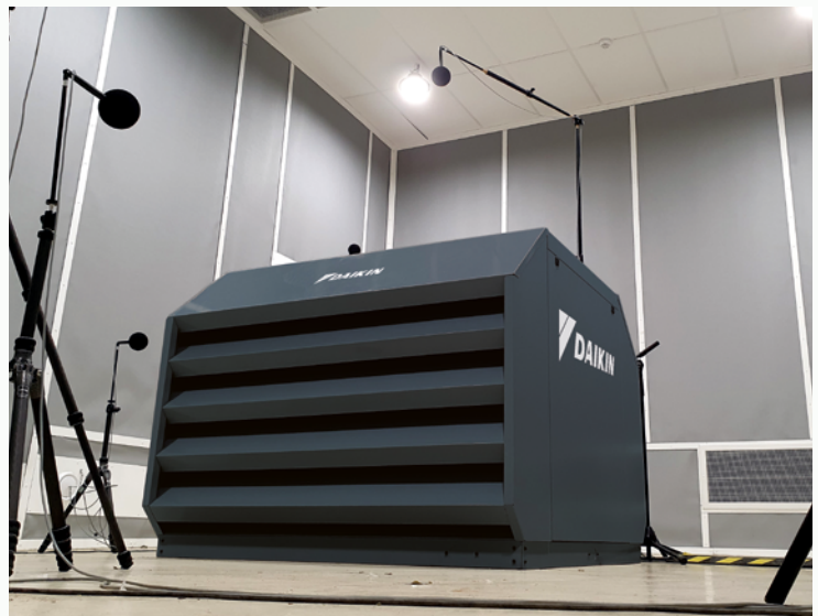
Sound power level measurement in acoustic chamber
