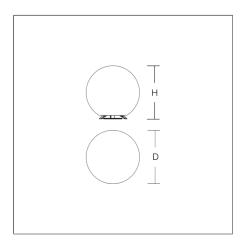
Decorative garden luminaire. Sphere can float in water and feature a flat base. Plastic base with opal plastic (polyethylene) diffuser sphere, satin finish. LED with colour change sequencer for battery operation - tuneable coloured light RGB or white. Light control via IR remote control. Full charge service life 8 to 12 hours (continuous operation). External charger for 100 - 240 V / 50 - 60 Hz with an inductive cradle included. Charge in dry rooms only!
