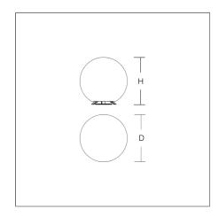
Decorative garden luminaire. Plastic base with opal plastic (polyethylene) diffuser sphere, satin finish. Fixture with pedestals and seperate adapter for fixed and ground-spike mounting. With 5 m connection cable including safety plug (Schuko), IP44. RGB lamp and accessory for ground installation must be ordered separately!
