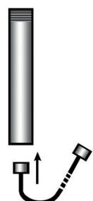
Pass the cable through the hollow pipe.
