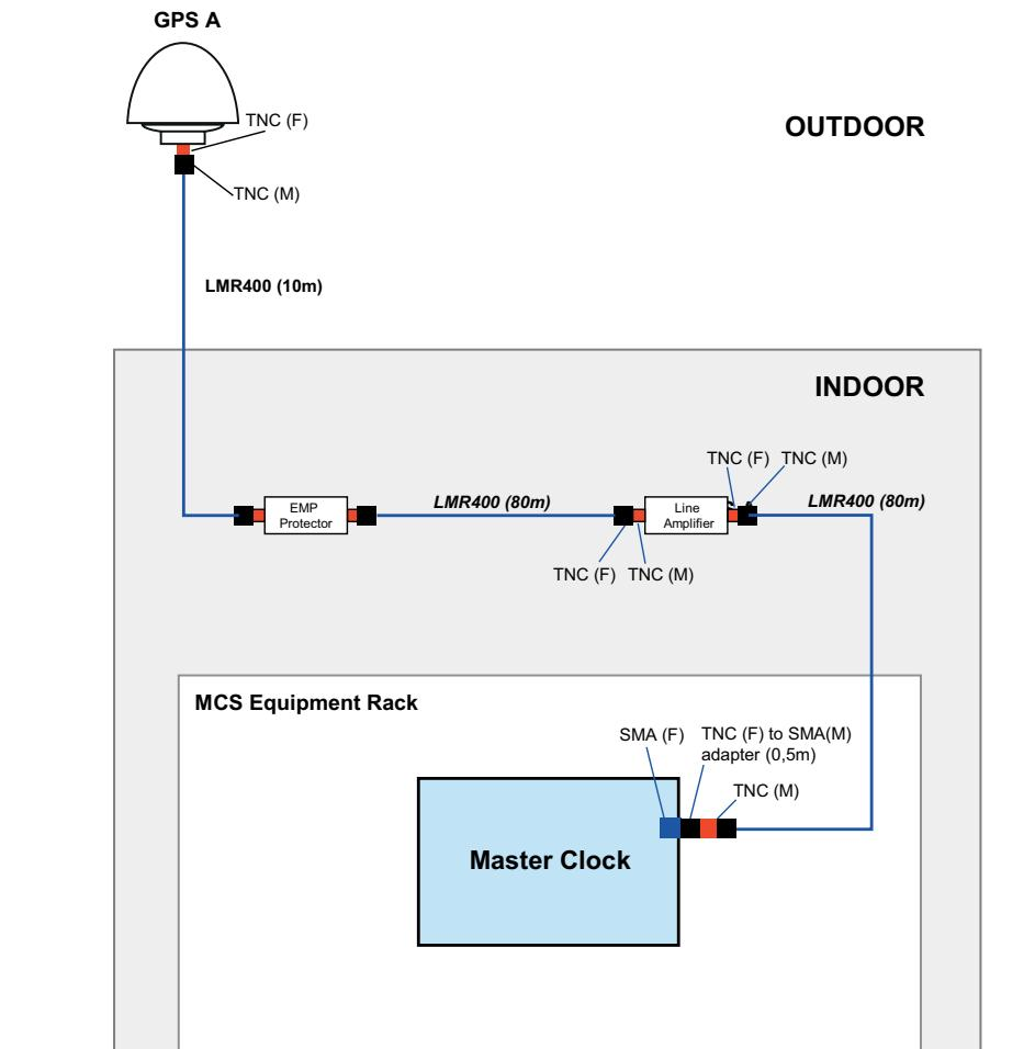
**GPS A** = BULLET III or HARDMOUNT GPS ANTENNA
