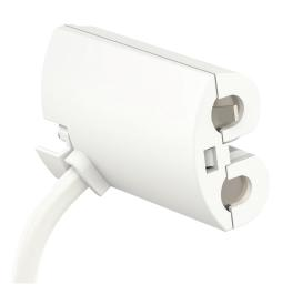
Danfoss Ally™ Power Module 24V is an accessory that connects the electronic radiator thermostat to an existing power system in the building and enables the device to work without batteries. The power output must be a 24 V supply from a safe source with a class II insulation level (Power supply with built-in double or reinforced insulation level between the supply voltage and safe voltage).
