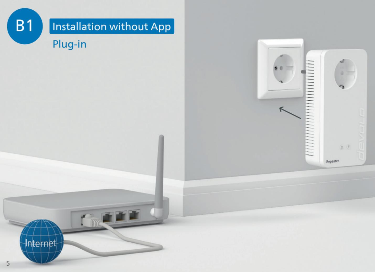
**| EN |** Plug the adapter into an available power socket and wait until the
