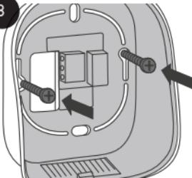
Fasten the thermostat's rear panel using the recess box screws.
