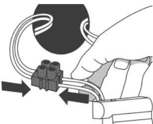
Connect the thermostat's power supply module cables to the power supply cables leading from the recess box, using an appropriate connector.
