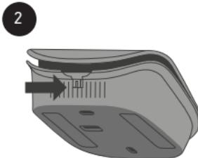
Unclip the front panel from the rear panel by pressing on the pressure point.
