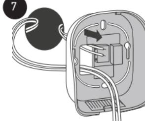
Feed the boiler control cables (NO / COM) through the rear panel.
