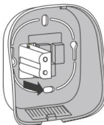
Feed the thermostat's power supply module through the orifice on the thermostat's rear panel.
