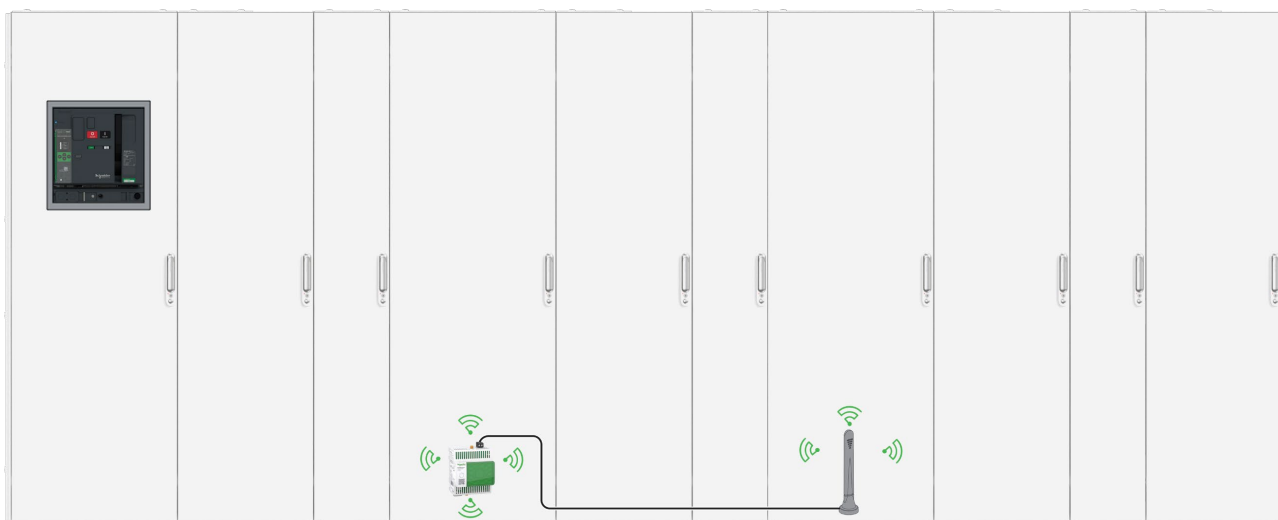
Illustration 5: Panel Server and antenna installation at the bottom of the column, covering seven columns
