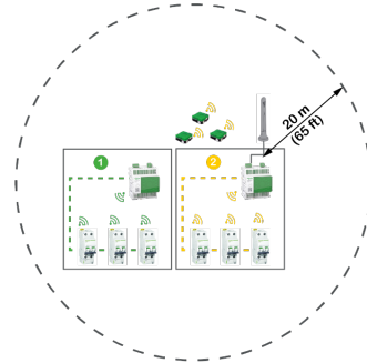
Installation with one concentrated wireless architecture
