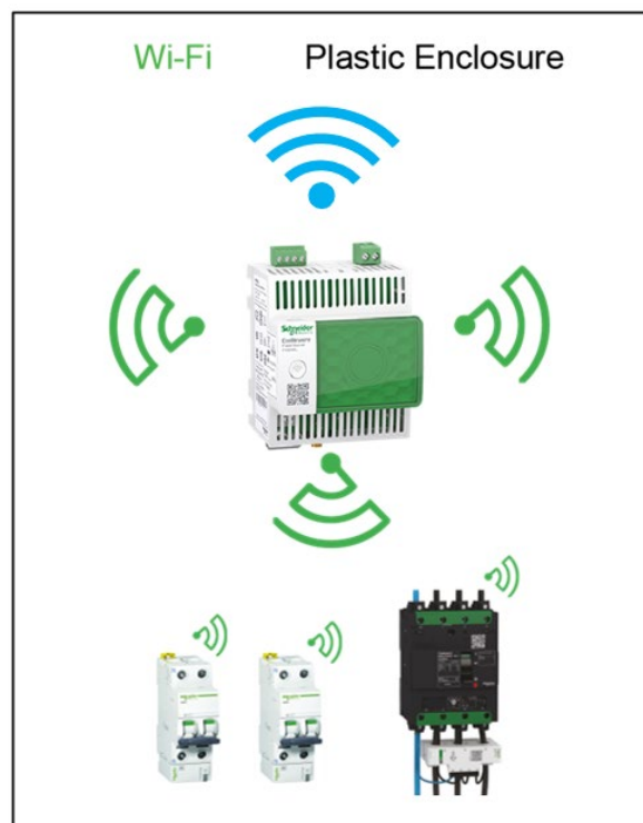
Illustration 9: Panel Server connected to Wi-Fi using internal antenna
