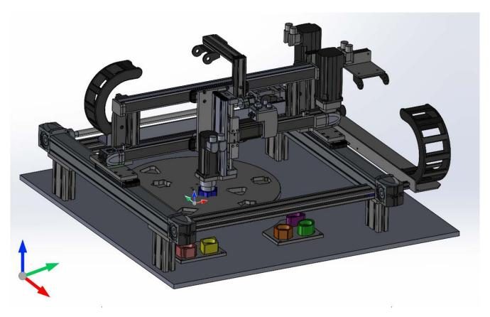
In the overall CAD file of the disk tracking machine, identify the parts that belong to the same axis of movement. Extract the selected parts and save each group to an individual CAD (Collada) file with the file extension \*.dae. For a list of CAD files that result from this disk tracking machine example, refer to Resulting CAD Files, page 19.
