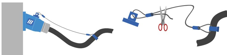
EYELET : Some handles are equipped with an eyelet. This eyelet allows an optimal pulling angle of the tension cord on the latch release mechanism.
