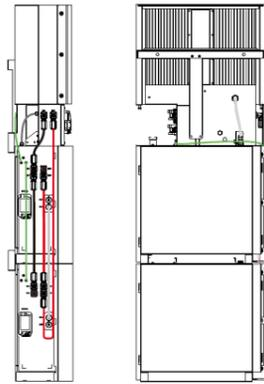
**Step 5** Close the battery covers and connect the PV-MC4 connectors to the system (connect ion on both sides).
