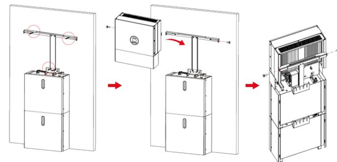
**Step 1** Hang the inverter onto the mounting panels, adjust the entire system and ensure that the battery and the inverter have been securely hung onto the panels and brackets.
