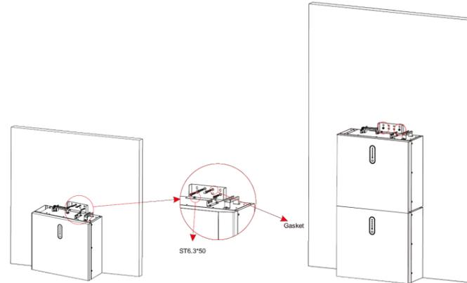
**Step 5** To assemble the second (and all other) battery, repeat steps 2 and 3 respectively.
