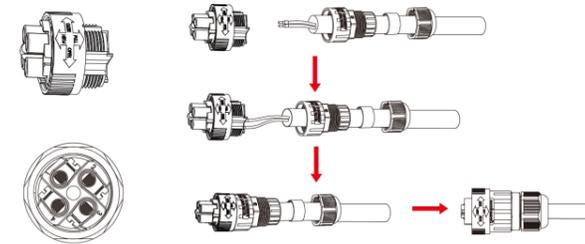
**Step 2** Install the waterproof component and screw on the waterproof sheath nut
