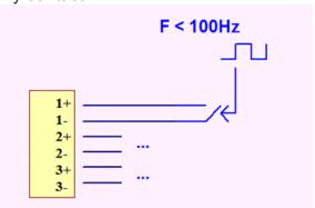
NPN Open Collector: compatible with voltage of 3V and a current of 3µA.
