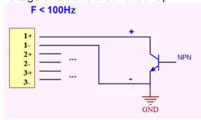
NPN Open Collector: Others, need to connect an compatible external power supply with a resistor to limit the current. Below exemple is given with an external 12V power supply.
