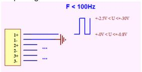
If there is no true 0Vdc for low state, then it is necessary to put a resistor between 1+/1- to make a pull down. The resistor could be a 100 kOhm.
