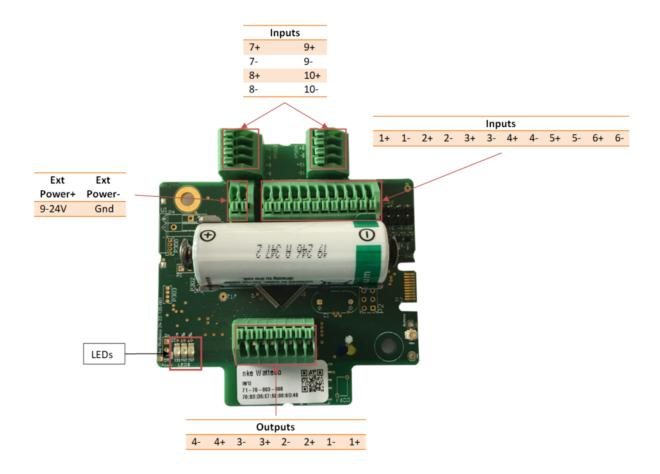
For the connectors, we recommend using several 20-26 AWG single wires. As the connectors pinch the wires plugged inside approximately 4mm from the wire end, strip the wires over a length of approximately 5 to 6mm before plugging them into the connectors.
