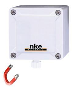
A reed switch is available under the sticker. A magnet can be used to activate it and perform specific actions on the sensor (switch off, switch on, reassociation...). When the reed switch is activated, the red LED blinks quickly.
