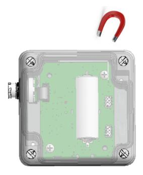
A reed switch is available under the "ILS" sticker. A magnet can be used to activate it and perform specific actions on the sensor (switch off, switch on, reassociation...). When the reed switch is activated, the red LED blinks quickly.
