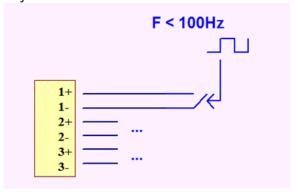
NPN Open Collector: compatible with voltage of 3V and a current of 3uA.
