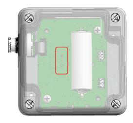
ASSN: blinking until the association with a network is done. Since release v3.5.2.5530, after 6 hours in association searching the led blinks all 1 minute.
