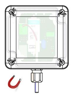
To switch off the device, repeat the same operation by placing the magnet next to the sensor for 5 seconds. After those 5 seconds, the red LED blinks 5 times slowly.
