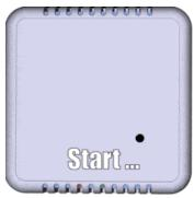
Each action can now be successively required by one more short pass with the magnet. The first short pass will show the current ABC calibration state: Blue => ABC ON; Orange ABC OFF. The next short passes will turn around the four following states:
