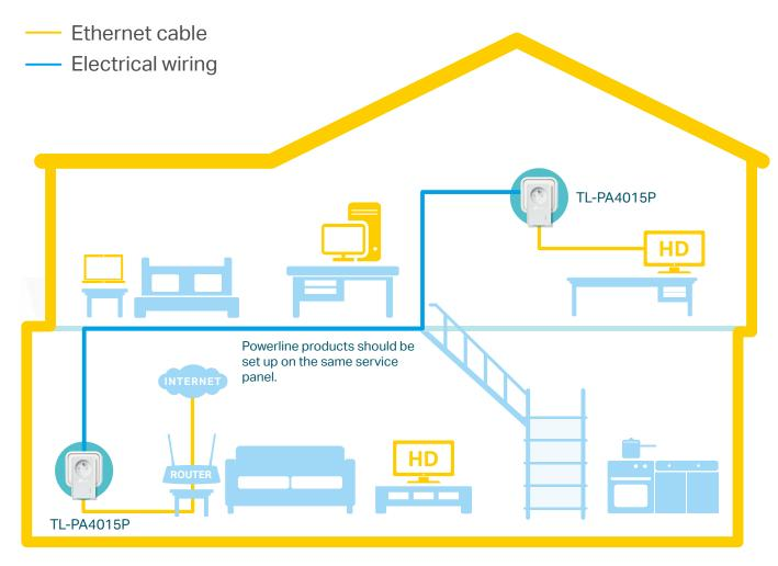
• No need for new wires or drilling • Network passes through walls and floors
