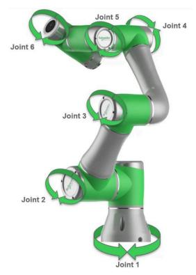
To add a gripper, right-click the **Cobot** assembly and execute the command **Tool Manager**. For further information, refer to *Managing Tools Within the* **Model** View in the EcoStruxure Machine Expert Twin Getting Started User Guide. To activate the gripper, connect the **Vacuum Actuator** signal of type BOOL to your controller. For status messages to the controller, connect the **Vacuum Sensor** signal of type BOOL.
