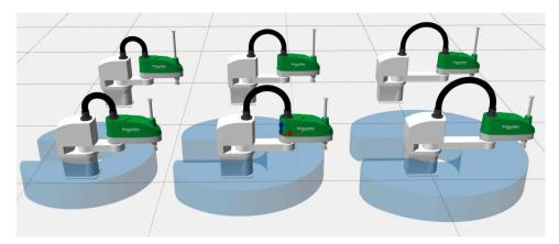
To add a gripper, right-click the **Scara Robots** assembly and execute the command **Tool Manager** from the contextual menu. For further information, refer to *Managing Tools Within the Model View* in the EcoStruxure Machine Expert Twin Getting Started User Guide. To activate the gripper, connect the **Vacuum Actuator** signal of type BOOL to your controller. For status messages to the controller, connect the **Vacuum Sensor** signal of type BOOL.
