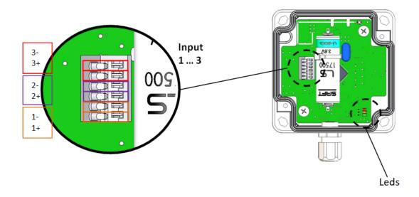
For the connectors, we recommend using several 20-26 AWG single wires. As the connectors pinch the wires plugged inside approximately 4mm from the wire end, strip the wires over a length of approximately 5 to 6mm before plugging them into the connectors.
