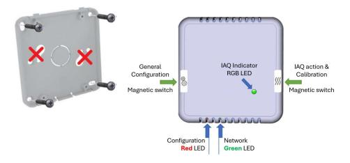
Once installed, the two LEDs are visible through the bottom vertical windows and the magnetic switches can be actuated like simple buttons using a magnet.
