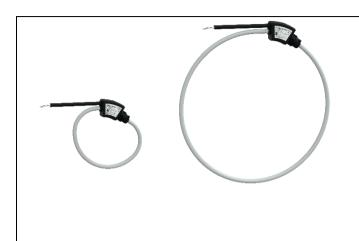
The CTRx Series of Rogowski flexible rope style Current Transducer provide secondary AC voltage proportional to the primary (sensed) current. These Rogowski coils are compatible with Schneider make EM35xxA, iEM35x5 and EM42xx series power meters.
