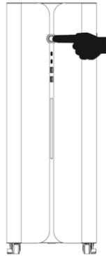
Once the unit has been properly installed and the batteries are connected well, simply press and hold the power button for 2-3 seconds till beep then release the power button to turn on the unit.
