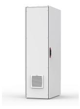
This outdoor vertical filter fan, EFP, with a polycarbonate cover and with a IP 55 protection degree, is easy to install thanks to its click-in feature. Unnecessary downtime is avoided, since water and dust are prevented from entering the enclosure through the filter, and the reliable fan motor will ensure constant ventilation. This filter fan is ideal both in indoor and outdoor environments, including direct sunlight thanks to its resistance to UV radiation.
