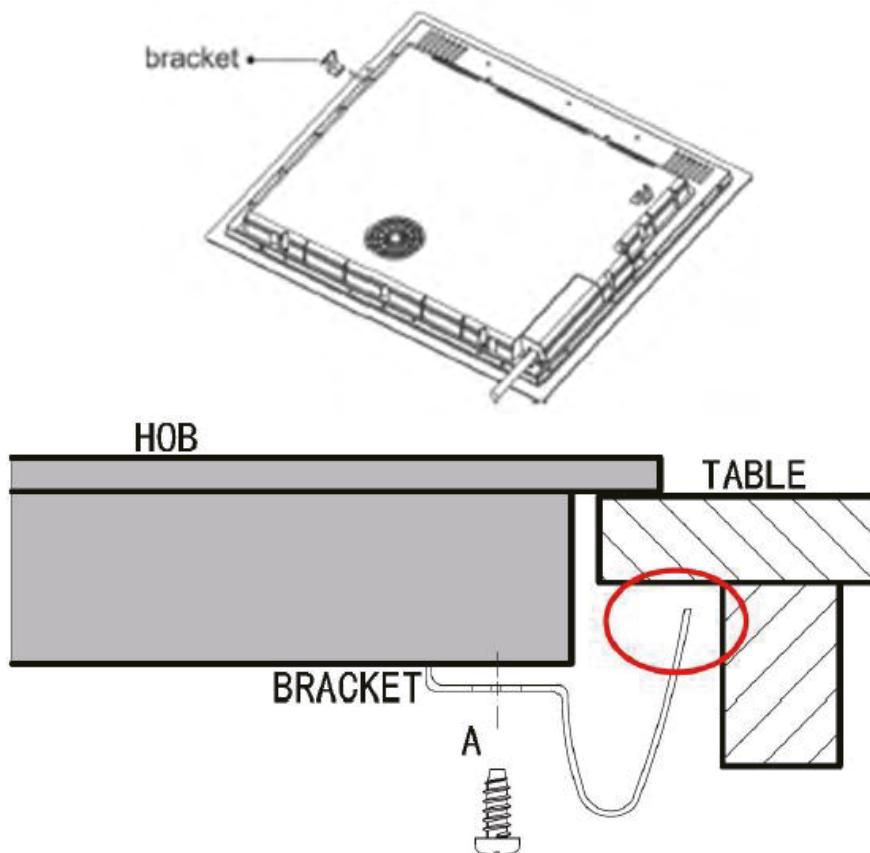
**⚠** Under any circumstances, the brackets cannot touch with the inner surfaces of the worktop after installation (see picture).
