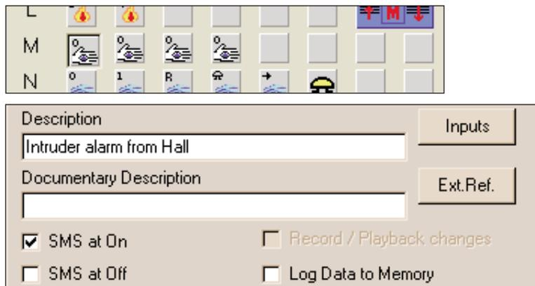
If the "SMS by ON" box is checked, the Mastergenerator will send an SMS with the time and date, the identifying text, the description text for the channel and the status, whenever E1 becomes active. The recipient of the SMS will see the following message in the display of the GSM phone:
