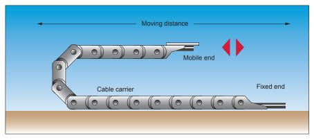
Cable carrier bending radius: approx.  $9 \times$  cable outer diameter
