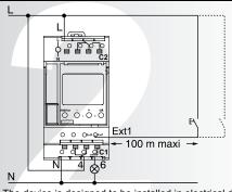
The device is designed to be installed in electrical distributions on a DIN rail (in accordance with EN 60715).
