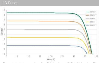
The module relative power loss at low light irradiance of 200W/m<sup>2</sup> is less than 3%.
