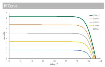
The module relative power loss at low light irradiance of 200W/m² is less than 3%.
