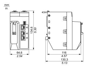
**NOTE:** Consider the height of the controller when you are planning the installation of the local rack. The controller extends below the lower edge of the rack by:
