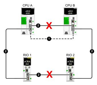
1 Hot Standby fiber optic link between CPU A and CPU B
