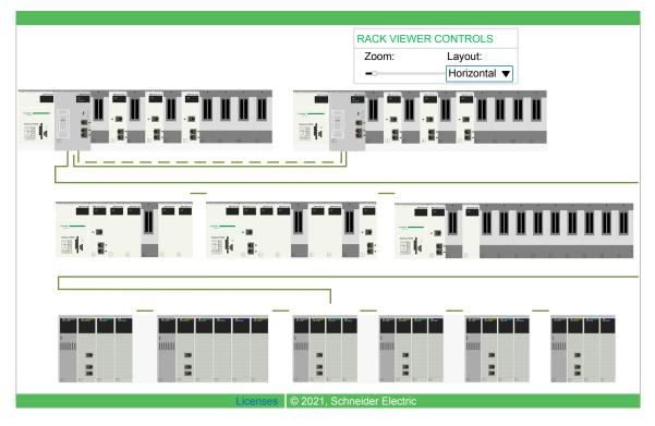
This example of a Rack Viewer page shows the Hot Standby connection between a primary CPU rack and a standby CPU rack. The Hot Standby connection (dashed line) is green when the Hot Standby link is healthy. If the Hot Standby link is not healthy, the dashed line is red.
