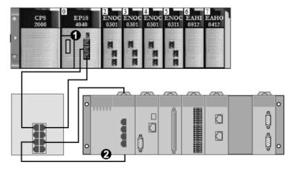
**1** M580 CPU: The CPU on the M580 local rack. In this example, you will enable this CPU's embedded scanner service as a local slave device (or target, **T**).
