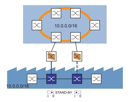
Figure 47: Transparent Redundancy
