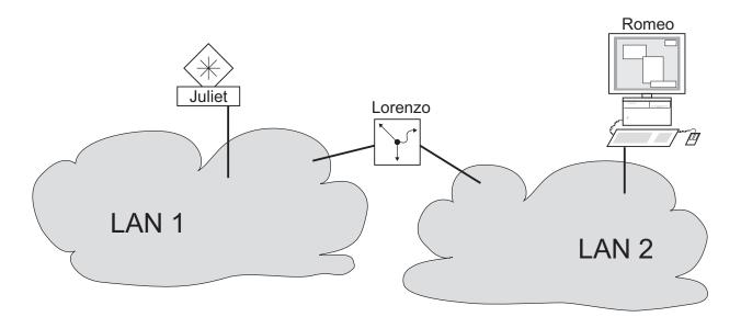
*Figure 9: Management agent that is separated from its management station by a router*
