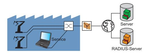
Figure 27: Application example for external authentication
