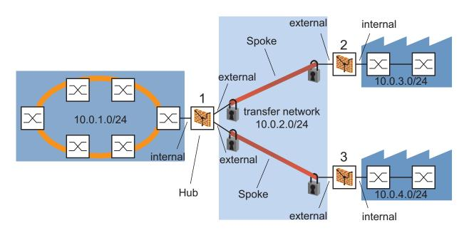
*Figure 42: Connecting several subnetworks via a public network (hub-and-spoke routing)*
