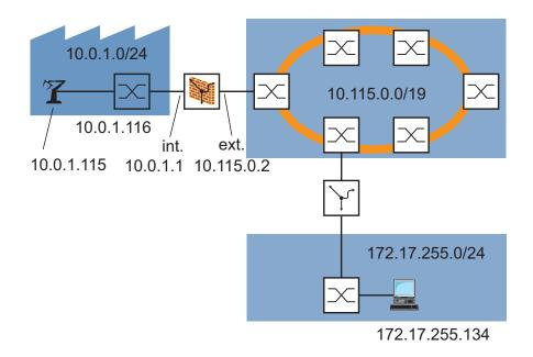
Figure 30: Firewall Learn Mode (FLM), application example
