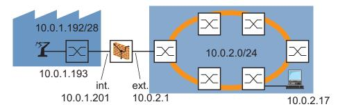
Figure 37: Managing a switch within the production cell from outside
