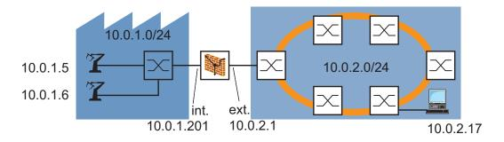
Figure 29: Packet filter with address template; application example
