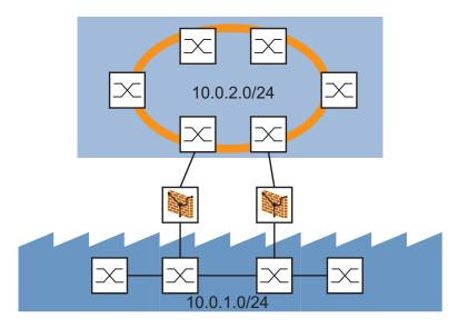
Figure 49: Router Redundancy
