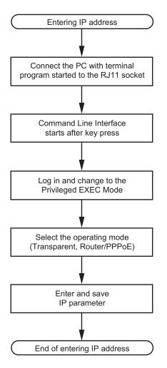
Figure 10: Flow chart for entering IP addresses
