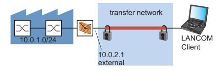
*Figure 45: Connecting a LANCOM Client with a private network via a public network*
