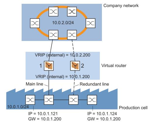
Figure 50: Router Redundancy application example
