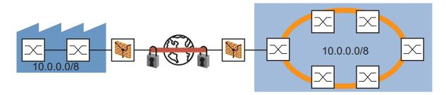
Figure 40: VPN for connecting two plant sections
