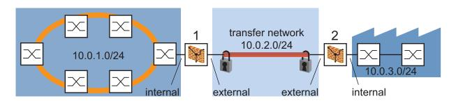
*Figure 41: Connecting two subnetworks via a transfer network*
