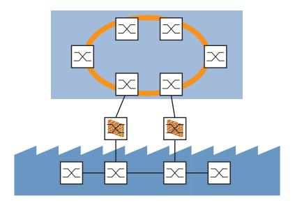
Figure 46: Redundant Firewall connection
