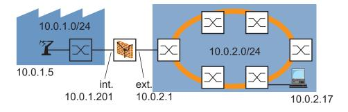
Figure 28: Application example for packet filter
