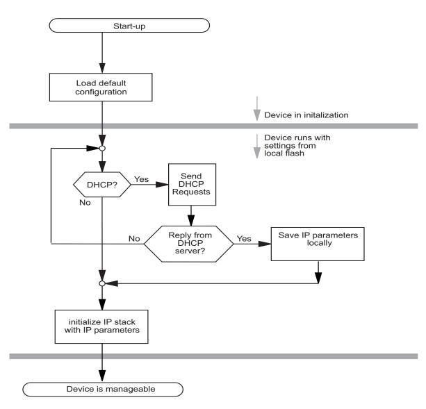
Figure 14: Flow chart for the DHCP process
