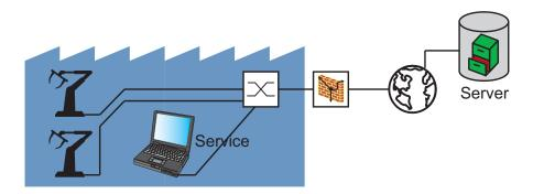
Figure 39: User firewall application example
