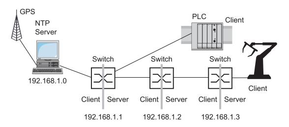
Figure 17: Example of SNTP cascade
