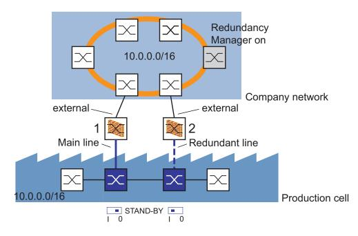
Figure 48: Transparent Redundancy application example
