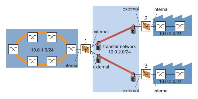
Figure 43: Addressing several identical subnetworks from a public network (Schneider Electric Address Mapping)
