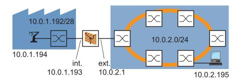
Figure 36: Connecting 2 Devices via Double NAT
